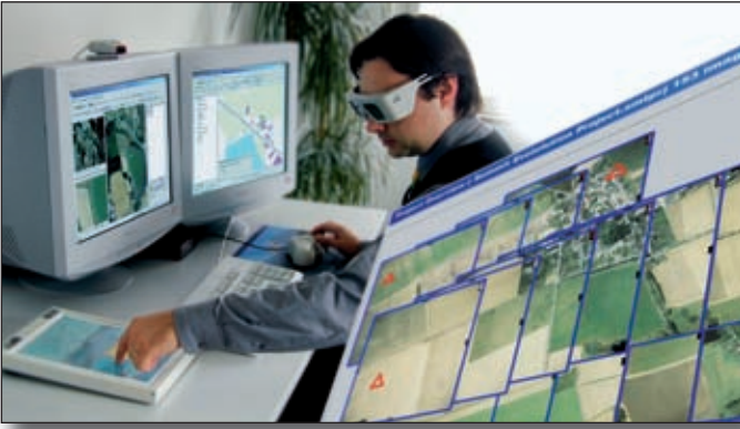
Fig. 3 –The Summit Evolution Digital Photogrammetric Workstation (DPW) that is used for feature data collection employing 3D stereo-viewing techniques.
